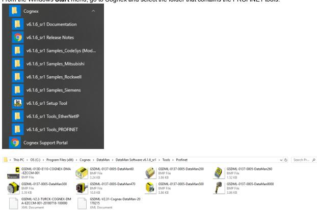
3. Check if the DataMan's firmware is up-to-date by clicking, in the Setup Tool, View and then System Info.
