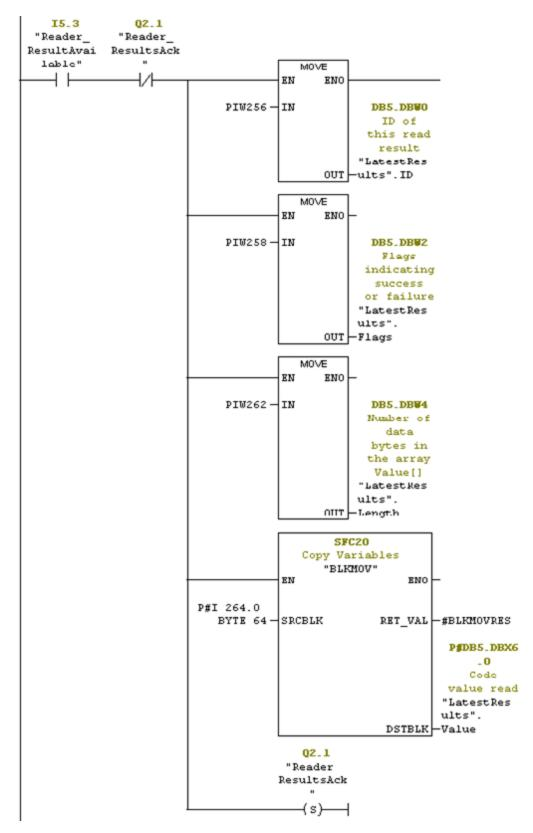
6. When the reader sees the result acknowledge signal, clear result acknowledge, clear the read pending coil, and signal that the read process is complete.
